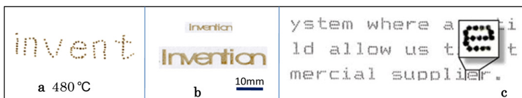
Fig. 4. Printing: (a) by the simulated heat-induced method, (b) by laser ablation, (c) by a dot matrix printer (Walker, 2008).
