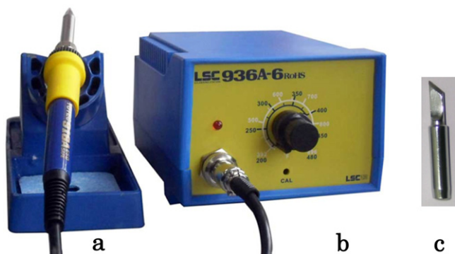
Fig. 1. An electric iron: its controller (a, b) and the shape of its head (a, c).
